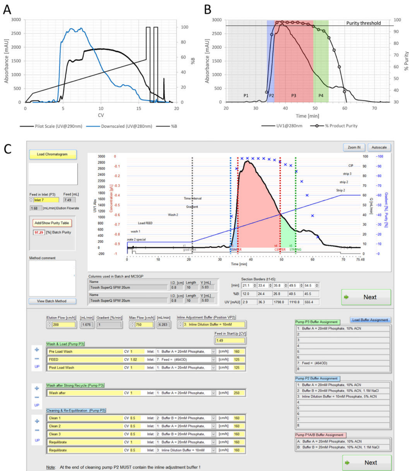
Figure 3. Single-column AIEC chromatographic profiles and the MCSGP design. (A) Black line: representative chromatogram of pilot-scale single-column batch production run showing absorbance UV@290 nm vs column volumes (CV) overlaid with %B modifier concentration (purification using the AKTA pure 150 M). The pilot-scale method was downscaled 78.6 \times and run on the Contichrom CUBE. (B) MCSGP design chromatogram. Absorbance UV@280 nm is overlaid with product purity (area% HPLC-UV). Product purity was measured by HPLC analysis, and each dot represents an analyzed fraction. Phases P1 to P4, as described in Figure 2B, are highlighted showing where MCSGP recycling and product collection boundaries were set. (C) - The MCSGP Wizard v8.1 software simplifies method creation.
