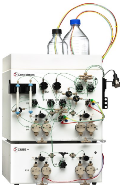
Fig. 5 Contichrom CUBE benchtop chromatography system
