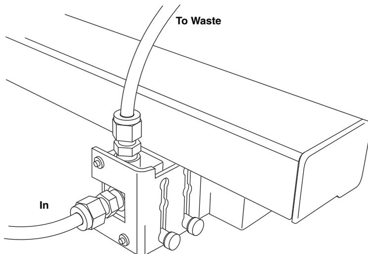
Figure 2-11 Connections to high flow diverter valve
