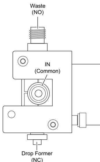
Figure 2-9 High flow diverter valve ports (front view)
