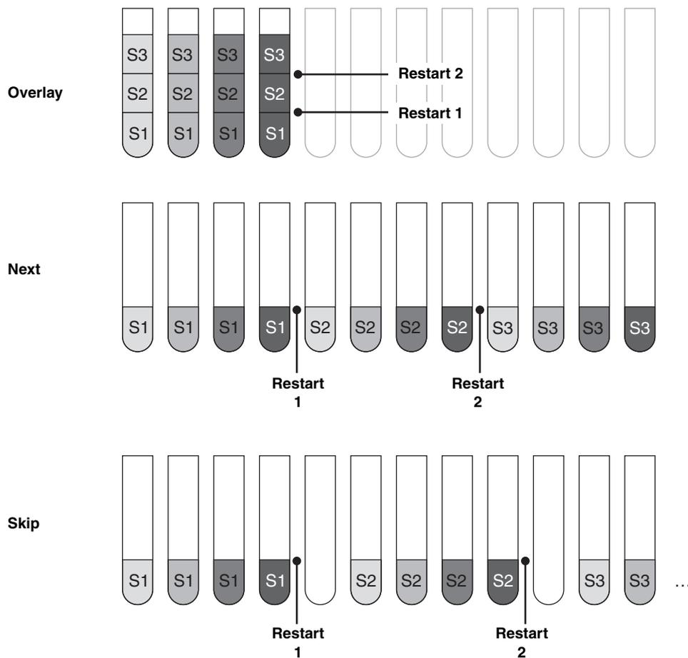
Figure 3-6 Overlay, Next and Skip options diagram
