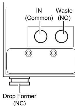
Figure 2-6 Diverter valve ports
