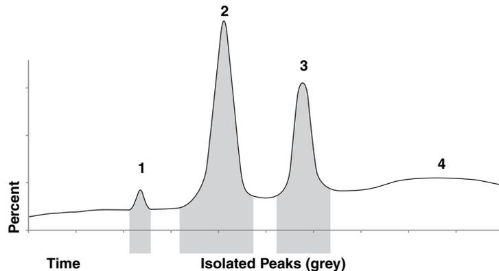
Figure 3-15 Peak Width detection cuts peaks when internal slope algorithms indicate a peak
